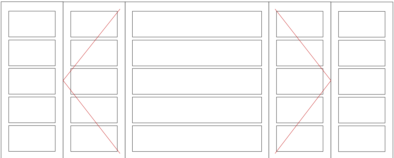
Front Elevation Ground Floor Bay – Lounge (5 sealed units, sub-divided by four rows of 22mm internal glazing bars)
